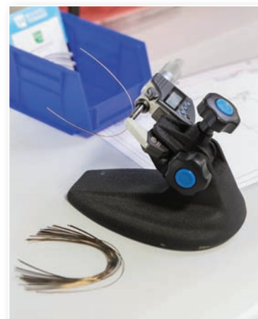
The diameter of all wires is tested for consistency of size.
