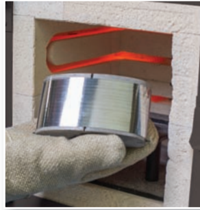
Heat-treatment sets the archform shape to wire.
