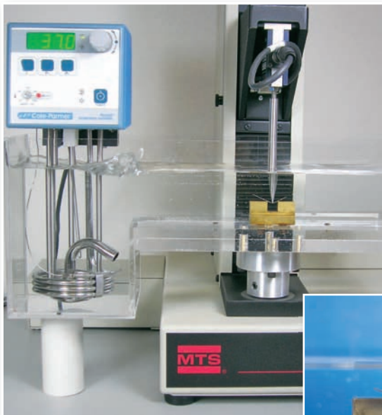
Waterbath force value and resiliency testing mimics intraoral environment.
