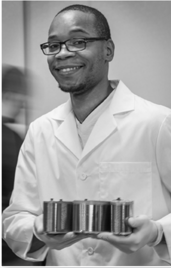
G&H employee, Jerome – Wire is wound onto precise forms of different sizes and shapes, then heat-treated.
